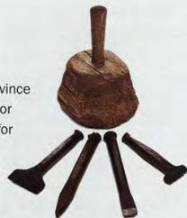
Well-used maul and selection of chisels: points for roughing out stone, toothed for shaping and modeling forms, and flat for finishing surfaces and details.
